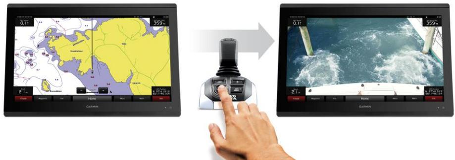
Certain boating functions, such as operating in reverse and using radar, require more focus. For example, by customizing information on layouts and linking them to the control and joystick, drivers can press an assigned button on the joystick which will bring up the docking camera view on the display.
